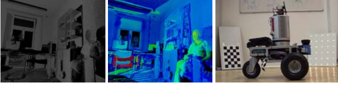
Fig. 1. Laser scan with reflectance (left) and thermal (middle) information. The robot Irma3D (right).
