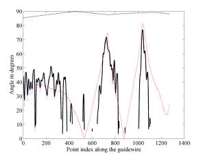
$\alpha$  is represented by a thin blue line;  $\beta$  is represented by a dotted black line; estimated  $\theta$  is represented by a thick black line; and true  $\theta$  is represented by a thin red line.
