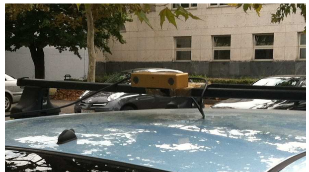
Fig. 1. The stereo system Bumblebee2 mounted on the car roof.
