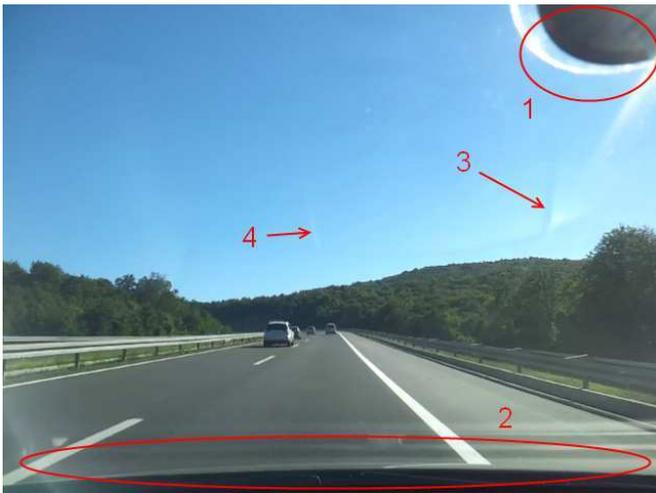
Fig. 1: A typical traffic scene. Note the camera mount (1), the dashboard (2), the reflection of car interior (3) and the speck of dirt (4)
