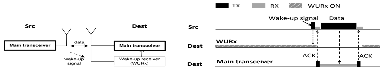
Figure 1. Implementing wake-up receivers on wireless sensor nodes
