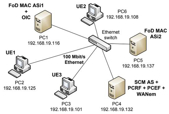
Fig. 5. Topology of the experimental testbed
