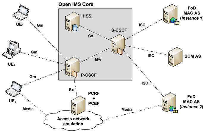
Fig. 2. Architecture of the IMS-based laboratory prototype
