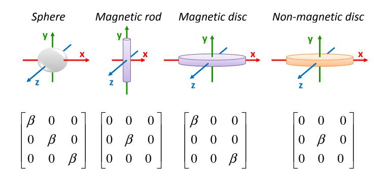
Basic principles of metallic target characterisation via magnetic polarizability tensor
