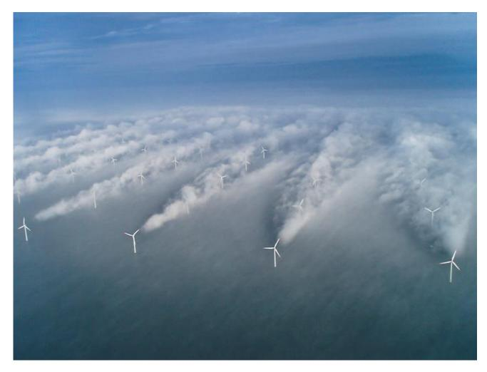
Horns Rev 1 wake effects. Photographer Christian Steiness. The above photograph shows the turbulence field behind the Horns Rev 1 offshore wind turbines
